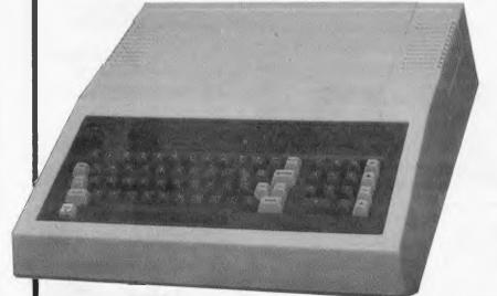
DUEL PROCESSOR 64K RAM-12K ROM 6502 & Z80a — Programmed Keyboard Upper & Lower Case — Joy Stick Port — Expansion Slots — Numeric Key Pad
