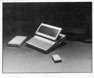
The Apple IIc personal computer with mouse, and large portable LCD display.
